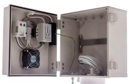
The AccelTex Solutions Heated & Cooled PoE enclosure allows an access point to be installed in an outdoor or other temperature-limiting environment. The heater, fan and AP are all powered by a single PoE cable run from the network switch. The enclosure ships ready for an AP installation with our 2.4/5 GHz 4/6 dBi omni antenna integrated onto the bottom of the enclosure.
